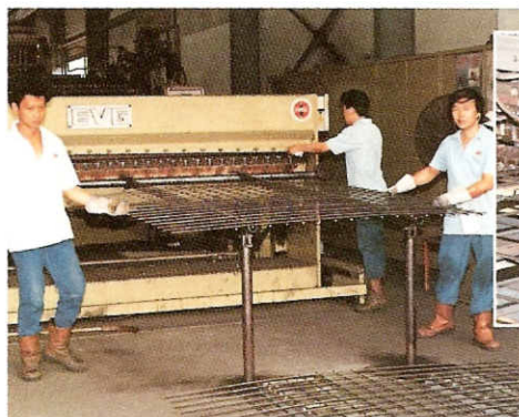
The G8 machine welds wires together to form mesh, at the rate of more than 75 welds per minute, and produces up to more than 60 tonnes of tailored mesh a day.
